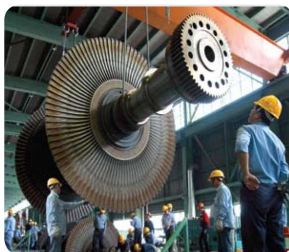
Steam turbine maintenance
